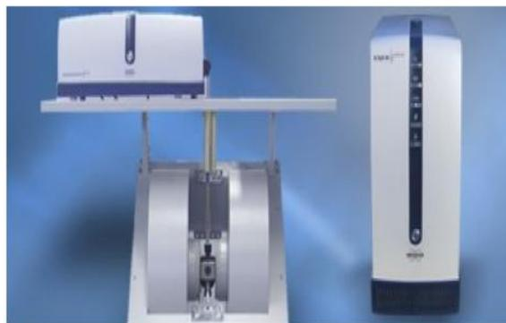
Electron paramagnetic resonance (EPR, Micro-EMX) for free radicals detection
